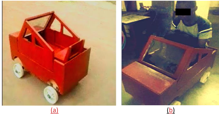
Figure 8: (a) Physical prototype of the ride-on toy car (b) testing the prototype using a subject of 62kg.
