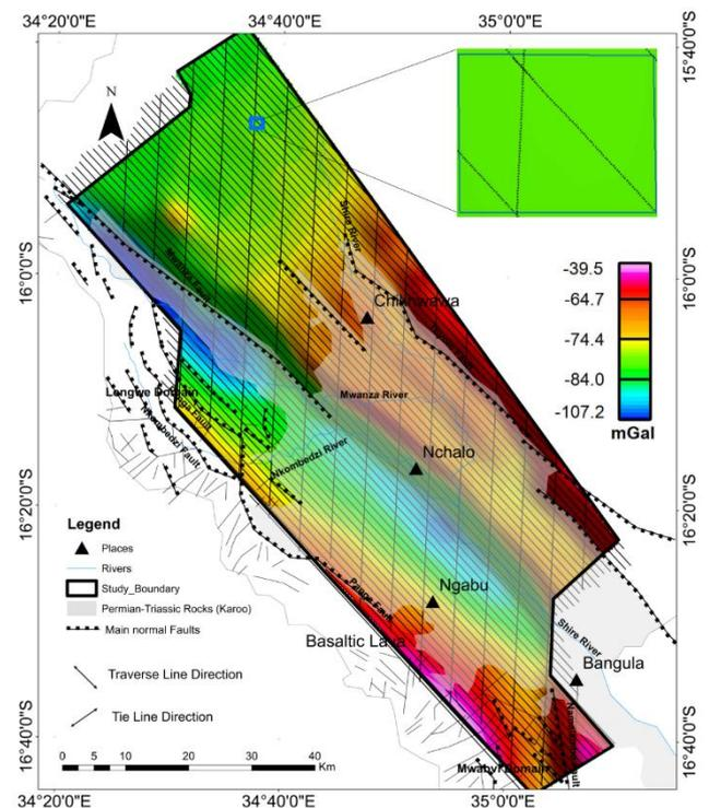
Figure 1: The gravity survey results showing the Bouguer anomaly map in the background, main existing faults, extent of alluvium deposition and data collection points with direction of traverse lines and control lines
